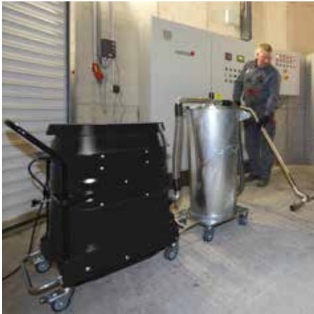
R01 A with pre-separator bin, 110 litres
